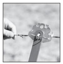
Attach the REEL-TITE to the handle and fasten with clip pin. Place the wire between the two pegs
